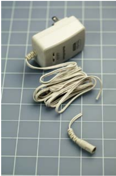
Figure 2-49. Preparing an AC adapter. First, cut off the little low-voltage plug and throw it away.
