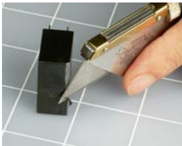
Figure 2-52. To look inside a sealed relay, shave the top edges of the plastic package with a utility knife til you open a thin crack.
