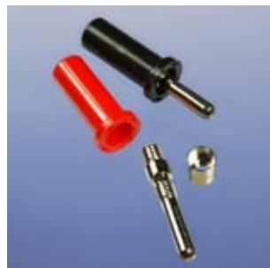
Figure 3-7. To make your own minigrabber meter leads, first attach a banana plug to a wire by sliding the wire through the cap, into the plug, and out through a hole in the side.
