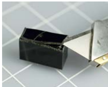
Figure 2-53. Insert the blade of your knife to pry open the top, then repeat the procedure for the sides.
