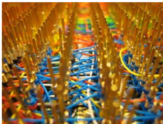
Figure 3-37. This picture shows some of the wire-wrapping in Steve Chamberlin's custom-built, retro 8-bit CPU and computer. "Back in the day," connecting such a network of wires with solder joints would have been unduly time-consuming and prone to faults. Photo credit: Steve Chamberlin.
