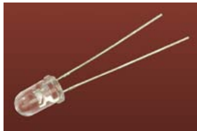
Figure 1-14. Typical 5-mm diameter light-emitting diode (LED).
