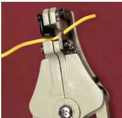
Figure 2-19. Using automatic wire strippers, when you squeeze the handles the jaw on the left clamps the wire, the sharp grooves on the right bite into the insulation. Squeeze harder and the jaws pull away from each other, stripping the insulation from the wire.
