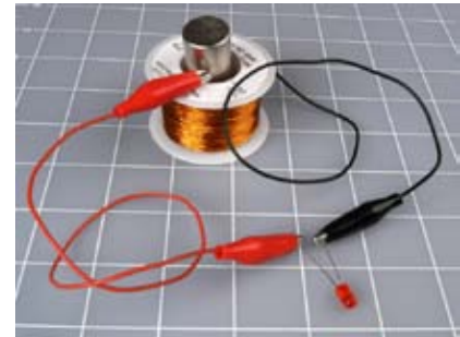
Figure 5-21. By moving a magnet vigorously up and down through the center of a coil, you generate enough power to make the LED flash brightly.
