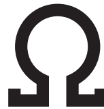
Figure 1-21. The omega symbol is used internationally to indicate resistance on ohms.
