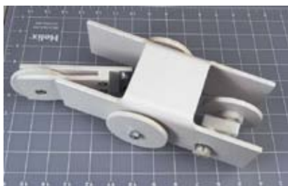
Figure 5-94. The assembled body of the cart, before adding control electronics. The wheel at the righthand end will pull the cart from left to right. The hinged trailing wheel will allow the cart to move in a relatively straight line when it moves forward, but will tend to turn it when it backs up.
