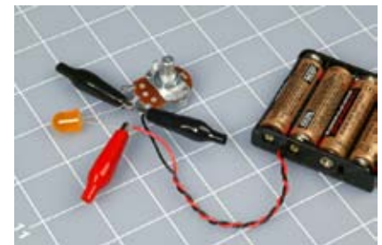
Figure 1-51. The LED in this photo is dark because I turned the potentiometer up just a little bit too far.
