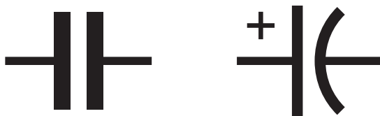
Figure 2-69. The generic schematic for a capacitor is on the left. The version on the right indicates a polarizing capacitor which requires its left plate to be “more positive” than its right plate. The plus sign is often omitted.
