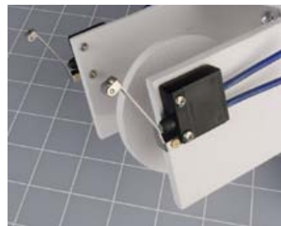
Figure 5-97. Two microswitches with metal arms are mounted on each side of the cart, where they will sense any obstacle.
