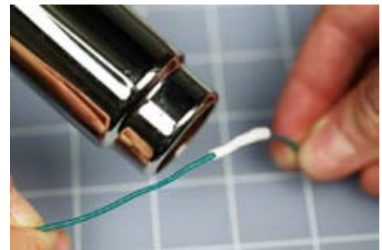
Figure 3-50. Leave the heat on the tubing until it shrinks to firmly cover the joint.
