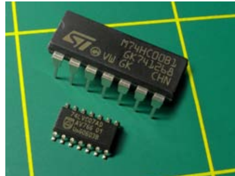
Figure 4-3. The DIP chip, at the rear, has pins spaced 1/10 inch apart, suitable for insertion in a breadboard or perforated board. It can be soldered without special tools. The small-outline integrated circuit (SOIC) surface-mount chip (foreground) has solder tabs spaced at 1/20 inch. Other surface-mount chips have pins spaced at 1/40 inch or even less (these dimensions are often expressed in millimeters). Surface-mount chips are designed primarily for automated assembly and are difficult to work with manually. In this photo, the yellow lines are 1 inch apart to give you an idea of the scale.
