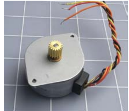
Figure 5-105. A typical stepper motor. The shaft rotates in steps when negative pulses are applied to four of the wires in sequence, the fifth wire being common-positive.
