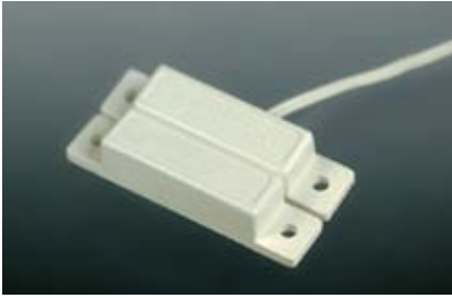
Figure 3-85. In this simple alarm sensor switch, the lower module contains a magnet, which opens and closes a reed switch sealed into the upper module.
