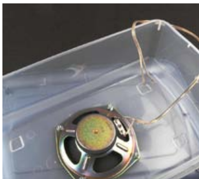
Figure 5-39. A resonant enclosure is necessary if you want to hear some bass (lower frequencies) from your speaker. A cheap plastic shoebox is sufficient for demo purposes.
