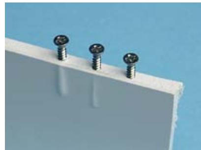
Figure 5-90. Three #4 screws driven into the edge of ABS, using a 1/16-inch guide hole, a 5/64-inch guide hole, and a 3/32-inch guide hole, respectively. Because the first two guide holes were too small, the plastic swelled around the screw (but did not break).
