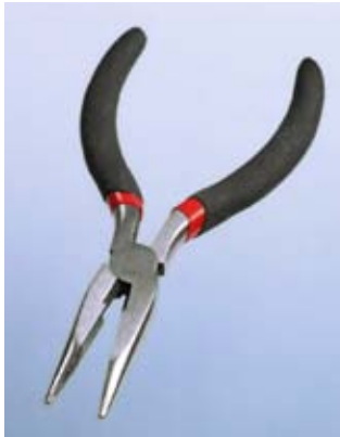
Figure 1-1. Generic long-nosed pliers are your most fundamental tool for gripping, bending, and picking things up after you drop them.
