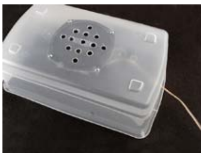
Figure 5-40. Drill some half-inch holes in the bottom of the box, then bolt the speaker in place, running a wire out through a hole in one end. Snap on the lid, and you're ready for not-quite-high-fidelity audio.
