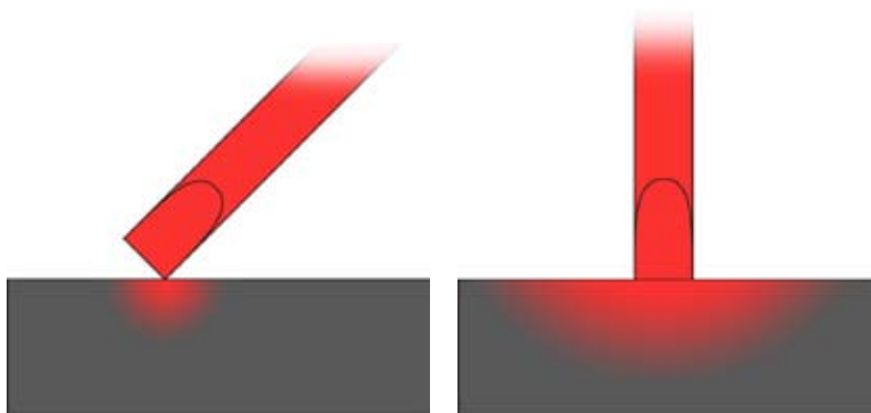
Figure 3-45. With only a small surface area of contact between the iron and the working surface, an insufficient amount of heat is transferred.
