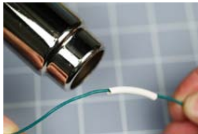
Figure 3-49. Apply heat to the tubing.
