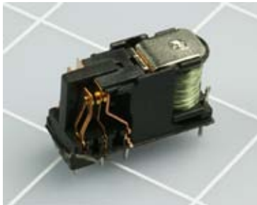
Figure 2-54. If you are really, really careful, the relay should still work after you open it.
