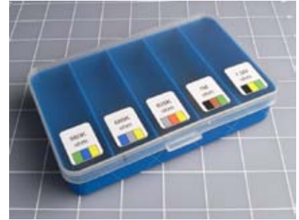
Figure 5-6. To check that resistors are not placed in the wrong compartments, print the color code on each label.
