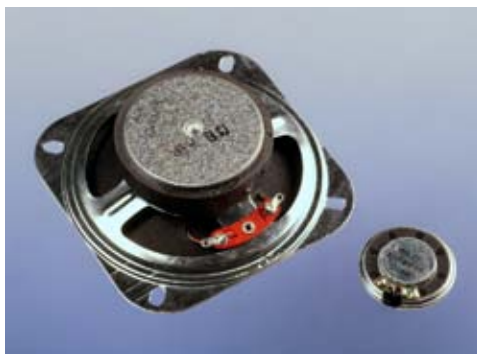
Figure 2-111. The 2N2222 transistor is quite capable of driving a 3-inch loudspeaker, which will create much better sound than a 1-inch speaker.
