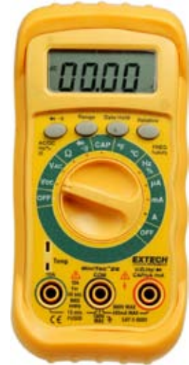
Figure 1-7. An autoranging meter from Extech offers basic functions, plus a temperature probe, which may be useful to check whether components such as power supplies are running unduly hot.
