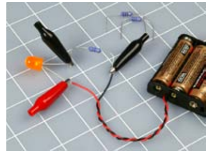
Figure 1-44. The setup for Experiment 3, showing resistors of 470Ω, 1KΩ, and 2KΩ. Apply alligator clips where shown, to make a secure contact, and try each of the resistors one at a time at the same point in the circuit, while watching the LED.
