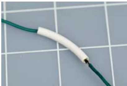
Figure 3-48. Slip the tubing over your wire joint.
