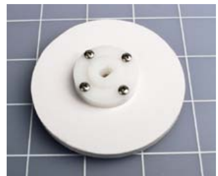
Figure 5-93. A 3-inch wheel is screwed to the disc that mates with the drive shaft of the motor.
