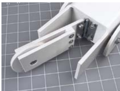
Figure 5-95. A closeup of the hinged trailing wheel, which rotates freely and can flip from side to side with minimal friction.
