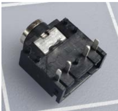
Figure 5-126. Closeup of the 3.5-mm stereo socket that is used with the USB download cable.
