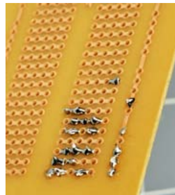
Figure 3-100. After soldering, the leads are snipped short and the joints are inspected under a magnifying glass. Another two or three components can now be inserted, and the process can be repeated.
