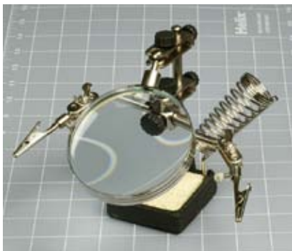
Figure 3-3. The helping hand is fitted with two alligator clips to hold your work. The metal spiral is a safe place to holster a hot soldering iron, and you use the sponge to wipe its tip.
