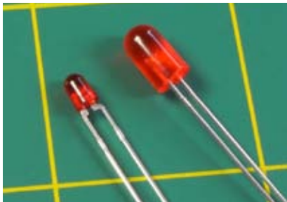
Figure 4-6. An HC series logic chip is rated to deliver only 4mA at each pin. This is inadequate to drive a typical 5 mm LED (right), which is rated for 20mA forward current. Miniature, low-current LEDs (left) will use as little as 1mA in series with a suitable resistor, and are ideal for test circuits in which you want to see the output with a minimum of hassle.
