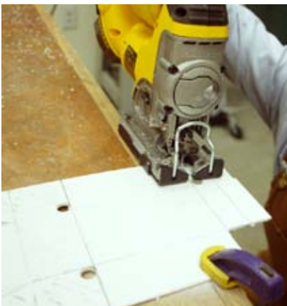
Figure 5-80. This DeWalt jigsaw can run at very slow speeds, enabling precise and careful work with plastic.
