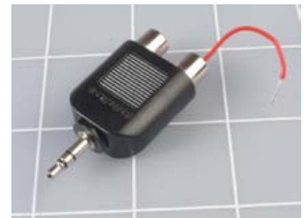
Figure 5-42. To sample the output from the headphone socket of a music player, you can use this adapter and push the stripped end of a piece of hookup wire into one of the sockets. Then use alligator clips on a jumper wire to connect the audio to your breadboarded circuit. Don’t forget to use an additional jumper wire to connect the outside of the socket to the negative side of the power supply on the breadboard. Because we’re only using one speaker, the amplifier is connected to only one of the stereo outputs from your player. The other is ignored.
